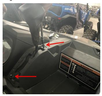
2.Place the bracket and fix it with the screws just removed, drill holes with a 3MM drill bit according to the screw holes on the edge of the bracket and fix it with screws, as shown in the figure:
