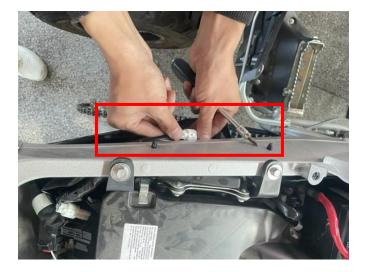
4. Install the new taillight in the same way as removing the original taillight, connect the wiring harness plug-ins (after the wiring harness is connected, start the vehicle to check whether it is powered on), and fix the taillight with screws after confirming that it can work
