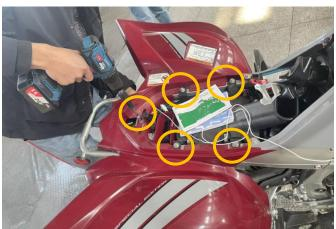
3. After the decorative board is removed, remove the two screws that fixed the original taillight, for later use, and unplug the wiring harness plug-ins of the original taillight, as shown in the picture:
