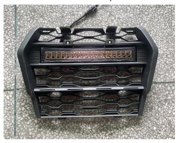
2. First, remove the original vehicle grille.As shown in picture:
