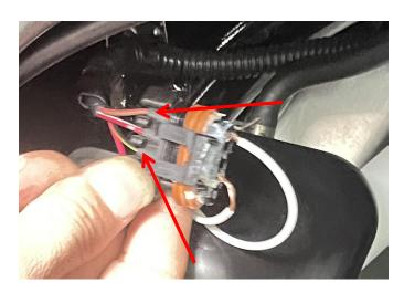
4. Pull the extension cable connected to the power supply along the gap to the grille, and connect it with the grille light, and then install the grille. As shown in picture:
