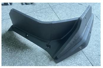
2. Unscrew the screws on the front fender flares of the original vehicle, and then install the assembled widened fender flares onto the original fender flares. Use the screws and nuts (M6 \* 30) provided with the product at the original screw holes to secure them again. As shown below:
