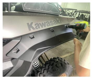
6. Prepare a 6mm drill bit, drill corresponding fixing holes according to the positioning holes on the widened fender flares, and fix them using the screws and nuts provided with the product (using M6 \* 30 screws). Assemble the other side in sequence according to the above steps. As shown below:
