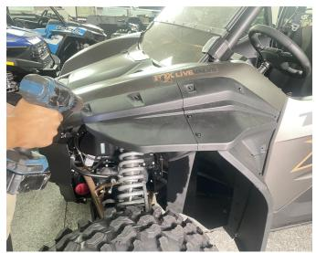
3. Prepare an 8mm drill bit, drill corresponding fixing holes according to the positioning holes on the widened fender flares, and fix them with nylon fasteners. Finally, use longer self tapping screws to fix the remaining screw holes. As shown below:
