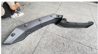
5. Unscrew the screws on the rear fender flares of the original vehicle, and then install the assembled widened fender flares onto the original fender flares. Use the screws and nuts (M6 \* 30) provided with the product at the original screw holes to secure them again. As shown below:
