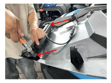
3. First, disconnect the spotlight wiring harness plug-in, facilitate subsequent wiring, and then connect the spotlight wiring harness to the vehicle running light wiring harness by
