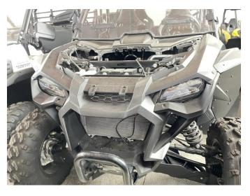
3. First, disconnect the wire harness of the grille light, and connect the latter half of the wire harness to the original vehicle's reserved extension wire harness using a broken skin method (black wire connected to green, red wire connected to white). The interface needs to be insulated and protected. Then, install the grille and fix it with the original vehicle screws. Finally, reconnect the newly disconnected wire harness. As shown in picture:
