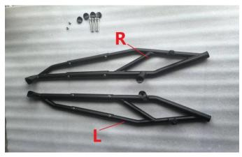
3. Remove the seat, the front end with two M10 \* 80 hexagonal screws, 2 castings, and the rear end with M10 nuts with washers from the inside through the frame to connect with the side bumper in three positions.
