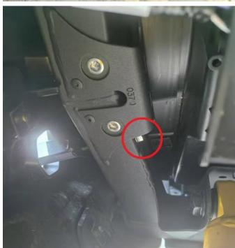
4. After tightening the 2 M10 screws at the front end and the M10 nut at the rear end, tighten all the connecting screws of the side bumpers, and the installation is completed.
