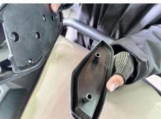
4. Mount the lamp on the back housing of the reverse mirror lamp, the lamp harness extends outside through the slots on the side, and finally reattach the mirror bracket, the mirror, and the outer compression frame (the other side of the reverse mirror is mounted using the same method).
