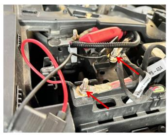
5. Will install the lights of the reversing mirror back to the vehicle, and then open the vehicle's original cover as well as the audio bracket, prepare the product supporting the control line, first of all, the power cord on the control line were connected to the positive terminal of the ACC junction box and the vehicle's battery light negative pole. As shown in the picture:
