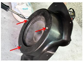
2. Remove the retaining screw from the vehicle's original side panel, then position the speaker pod in the properly aligned location and reinstall the original screw. Finally, secure the pod by driving the included self-tapping screws into the corresponding mounting holes in sequence. (Repeat the same procedure on the opposite side) as illustrated:
