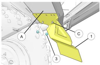
3. Using LH mudflap ① as template, drill two holes on floor panel (A) and two holes on rocker panel (B) at driver's side of the vehicle as shown.
