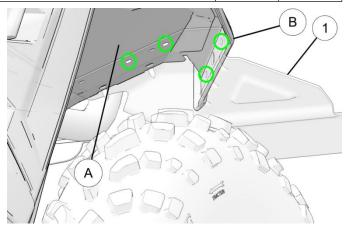
4. Fix the LH mudflap ① by installing four tuflok rivets⑤ and washers ④ as shown.
