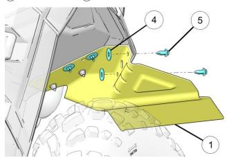
5. Repeat Steps 2-4 to install the RH mudflap ② on passenger side of the vehicle.
