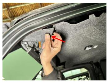
3. Peel back the roof liner and position the sun visor mounting bracket onto the vehicle frame (aligning the bracket's screw holes with the pre-drilled holes on the frame). Then secure
