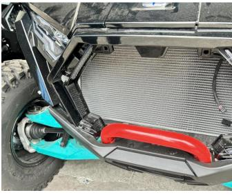
3. Take out the new accent light, re-connect the wiring harness plug-ins of the new accent light, and then use the matching iron nuts to fix the new accent light on the original vehicle (the other side can be replaced and installed in the same way), and finally reinstall the original front grille of the vehicle. As the picture shows:
