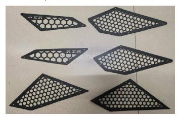
2. Compare the positions of the mounting holes with the protective cover, and then drill mounting holes with a diameter of 3.2mm one by one, as shown in the picture:
