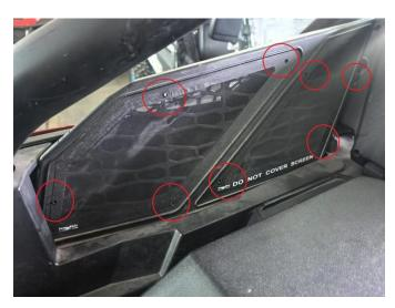
3. Assemble 6 pieces of protective covers onto the air intake filter screens one by one with 24 self-tapping screws of M4\*12, and then the installation is completed.
