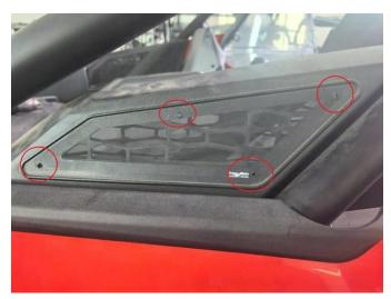
3. Install the protective covers onto the protective nets with 8 self-tapping screws of M4\*12, and then the installation is completed.
