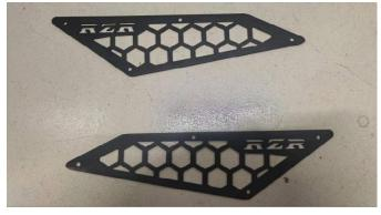
2. Compare the positions of the mounting holes with the protective cover, and then drill mounting holes with a diameter of 3.2mm one by one, as shown in the picture:
