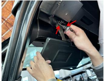
3. After the installation is completed, you can reinstall the roof lining and tighten the fixing screws. Finally, adjust the tightness of the sun visor by adjusting the screws. As shown in the picture:
