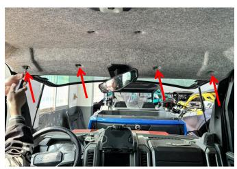
2. Lift up the roof lining, find the screws reserved for fixing the sun visor on the original vehicle. After loosening the nuts, install the sun visor bracket onto the screws, and then screw the original nuts back in place (install the other side in the same way). As shown in the picture:
