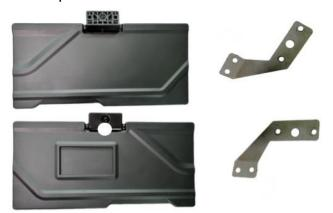
1. Assemble the sun visor and the mounting bracket together by using the matching screws. Then, get into the driver's cab and remove the screws that fix the roof lining. As shown in the picture:
