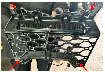
4. Use the adapter cable for the new mesh grill, pull the adapter cable from the mesh grill to the headlights and daytime running lights through the gap under the vehicle, connect the adapter cable for the mesh grill spotlights to the headlight harness plug-in, connect the adapter cable for the daytime running lights on the mesh grill to the original daytime running light harness plug-in, and then finally install the new mesh grill to the vehicle.
