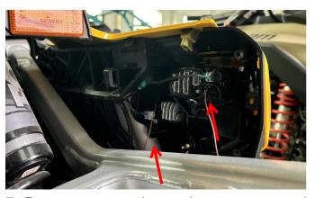
7. Prepare an extension cord, connect one end to the daytime running light harness on the new headlights (the connection needs to be well insulated and protected), pull the extension cord through the gap to the vehicle's ACC power supply, and connect the extension cord to the ACC screw post, and then finally install the previously disassembled decorative panels, hoods, and the mesh grille back to their original positions.
