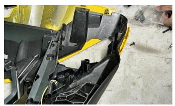
5. Move the rubber ring and adjusting screw on the original headlight to the new headlight according to the original position, and then install the new headlight to the front fascia, and use the original screws to fix it. (The other side of the headlamps can be replaced and installed in the same way.)
