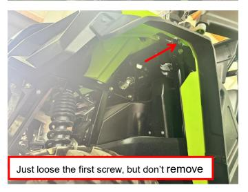
4. Install the assembled mirror unit to the vehicle: Hook one end of the mirror bracket onto the screw that was just loosened, and secure the other end with the original A-pillar screw. After adjusting the angle of the side
