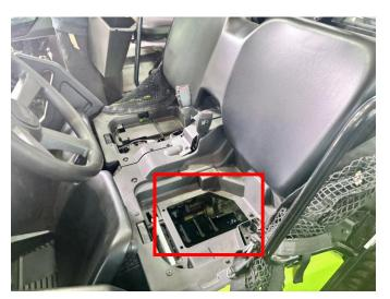
3. Place the storage box in the groove, then use the M8 drill bit to drill holes according to the corresponding screw holes on the storage box. Finally, fix it with the snap fasteners and reinstall the seat cushion. As shown in the figure:
