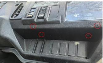
3. Secure the cup holder bracket under the instrument panel using four self-tapping screws. Then, attach the cup holder to the bracket to complete the installation.
