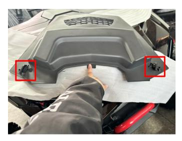
2. Install the new hood onto the vehicle and tighten the locking buckle. As the picture shows:
