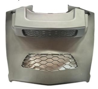
1. First, remove the original vehicle hood and install the fixing wrenches and rubber plugs on both sides onto the new hood. As the picture shows:
