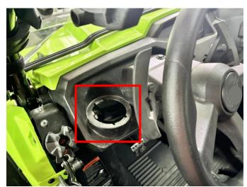
3. Install the new cup holder onto the vehicle. When installing, the notch on the new cup holder should be aligned with the slot on the vehicle. Then, press down firmly to fix it (the other side can be installed in the same way). As shown in the figure:
