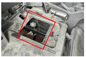
3. First install the large storage box, and then install the small one. Then, use an 8MM drill bit to drill holes on the vehicle according to the corresponding positions of the fixed holes on the storage box. Finally, fix it with the nylon clips that come with the product. As shown in the figure:
