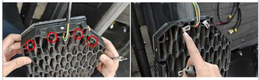
• Align the DRLs with the holes on the grille edge and secure them using the L-shaped spacers (Accessory (5)) and M3 self-tapping screws (Accessory (6)).
