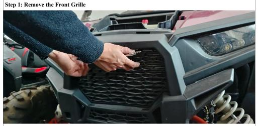
• Release the 2 upper tabs on the grille, tilt it outward slightly, then lift to disengage the lower tabs and remove the grille.
