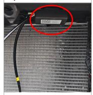
Peel off the adhesive backing and attach the controller to a suitable location.
