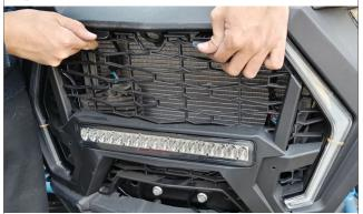
• Release the 2 upper tabs on the grille, tilt it outward slightly, then lift to disengage the lower tabs and remove the grille.
