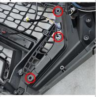
Remove 3 nuts (fig.upper) from the original DRL; replace with new DRL and secure.
