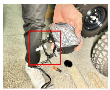
2. Unscrew the two fixing nuts at the A-pillar of the original vehicle, and add one aluminum lining tube for the spotlight on each of the two screws. Then install the spotlight bracket, adjust the angle of the spotlight, and use the original vehicle nuts to lock it. As shown in picture:
