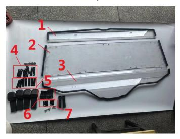
1. Assemble the PC boards with 14 M6\*20 socket head cap screws, 7 brackets #4 and 7 brackets #5, and install bracket #4 on the outside. As shown in picture:
