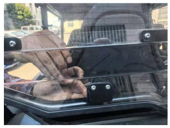
3. Secure the rear windshield to the rear post of the frame with four large straps and two small straps and complete the installation.
