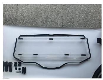
2. Put the rear windshield to the rear of the frame according to the position shown in the picture, and then fix the lower end of the rear windshield to the rear frame with four M6\*20 hexagon socket head cap screws, four M6 anti-loosening nuts, and two brackets #6 and two brackets #7. As shown in picture:
