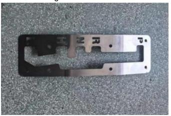
3. Unscrew the shift lever head and use seven M4\*10 self-tapping screws to secure the stainless steel panel to the vehicle's original plastic panel. Tighten the screws and ensure that the panel is flat and flush.
