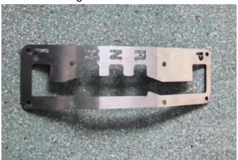
3. Unscrew the shift lever head and use eight M4\*10 self-tapping screws to secure the stainless steel panel to the vehicle's original plastic panel. Tighten the screws and ensure that the panel is flat and flush. Installation complete.
