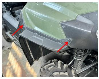
4. Prepare a 6mm drill bit. Drill holes along the fixing holes on the fender flare at the corresponding positions on the vehicle (only two fixed holes need to be drilled). Then, use the matching M6 screws, nuts and M4 self-tapping screws to fix them (install the other side in the same way). As shown in the figure:
