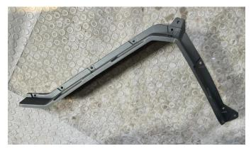
3. Pry out the two pins on the vehicle. Place the assembled fender flare on the vehicle, and then press the pins that were just pried out back into their original positions to fix the fender flare. As shown in the figure:
