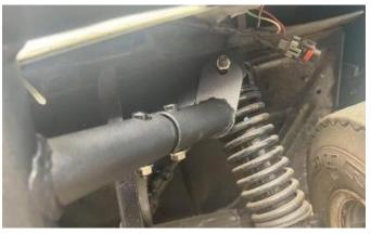
7. Install the lower end of the front bumper to the lower front of the frame with two M10\*65 external hexagon screws with washers and two M10 lock nuts, as shown in the figure. Tighten all the screws and nuts. The installation is completed.
