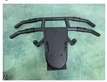
5. Remove the two nuts that connect the plastic part at the lower end of the golf cart and take off the plastic part.
