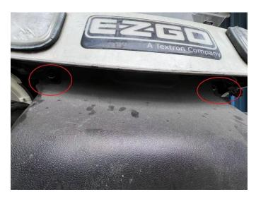
6. Install the upper end of the front bumper onto the front frame with two M10 lock nuts, as shown in the illustration:
