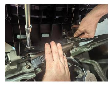
5. Fix the bracket on the front rack cover with two pins and complete the installation. As shown in the figure:
