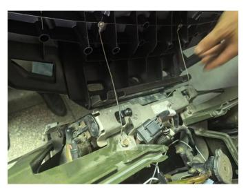
3. Remove the pins on the bracket and then take off the bracket.
