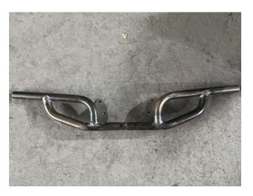
3. Then, install the rear bumper onto the rear frame with four M8\*20 flange external hexagon self-tapping screws. Tighten the screws and complete the installation, as shown in the illustration:
