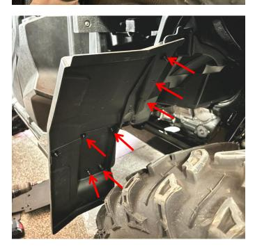
4. Position the other mudguard at the edge of the rear cargo. According to the mounting holes on the mud guard, drill holes at corresponding positions on the vehicle body using a 6mm drill bit. Secure them with screws and nuts. Finally, reinforce the bottom section of the mudguard using retainer clips and self-tapping screws. (Repeat the procedure identically for the opposite side.) As illustrated:
