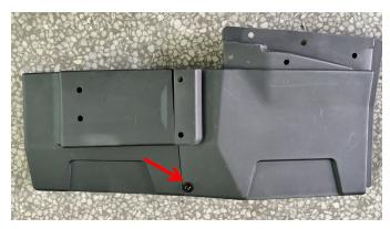
3. Open the rear cargo door of the vehicle. First, position the rear mudguard in its designated location on the vehicle. Prepare a 6mm drill bit, and drill holes on the vehicle body corresponding to the mounting holes on the mudguard. Secure it using the provided screws and nuts. As shown in the figure:
