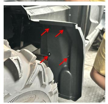
4. Attach the other assembled mudguard to the iron bracket of the vehicle accordingly. Then,
