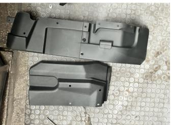
3. Open the rear cargo gate, first place the single-piece mudguard against the side of the vehicle's step plate. Then prepare a 6mm drill bit and drill holes in the vehicle according to the fixed hole positions on the mudguard. After that, secure it using the provided screws and nuts. As shown in the figure:
