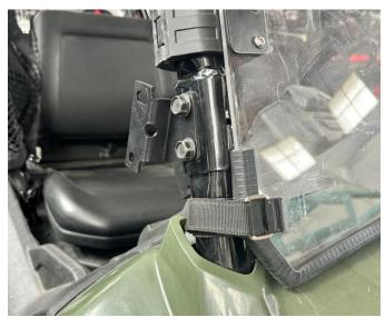
3. Use the screws and nuts in the package to fix the side mirror onto the bracket (Install the other side in the same way). As shown in the figure:
