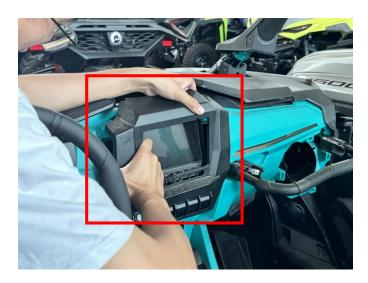
2. Remove the original instrument panel. As shown in the picture:
