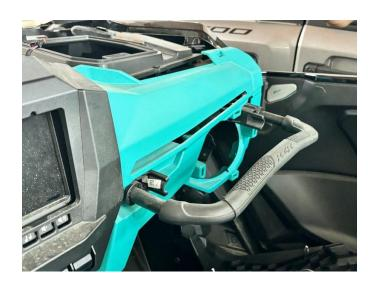
Connect the wire harness with the terminal copper round to the original vehicle terminal post. Then, unplug one reserved expansion plug-in on the original vehicle, and connect the corresponding wire harness plug-in on the adapter cable with it. Finally, connect the remaining two types of wire harness plug-ins with the dash lights respectively. After completion, install the previously removed parts back to their original positions. As shown in the picture:
