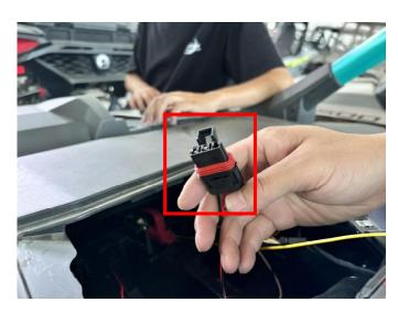
4. For vehicle models that do not have original dash lights in the original vehicle, we have an extra adapter cable. The specific installation operations are as follows: Prepare the adapter cable matched with the product.
