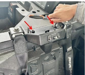
2. Remove the original-sized audio speaker and reinstall it on the new speaker pod. Fix it with self-tapping screws. Install the matching clips on the outer frame of the speaker pod. After that, press and fasten the outer frame onto the rear shell of the speaker pod. As
