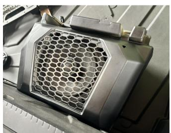
3. Thread the wiring harness of the speaker pod through the wiring hole. Then, snap the new speaker pod onto the iron bracket below.
