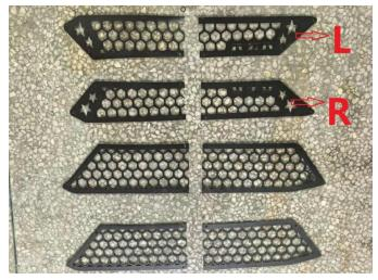
1. Fix the outer intake cover (with letters) to the outer frame of the intake filter with 4 self-tapping screws of 4\*12, as shown in the picture:
