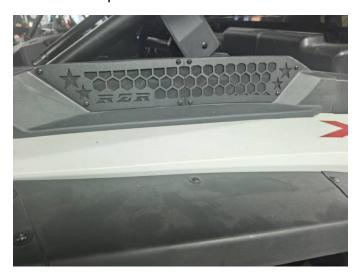
3. Install the inner intake cover onto the outer frame of the inner filter with 4 self-tapping screws of 4\*12, as shown in the picture:
