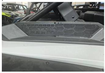
2. Install the other end onto the outer frame with 4 self-tapping screws of 4\*12, and ensure the connection positions are aligned neatly, as shown in the picture:
