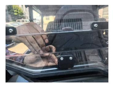
3. Secure the rear windshield to the rear post of the frame with two large straps and two small straps and complete the installation.
