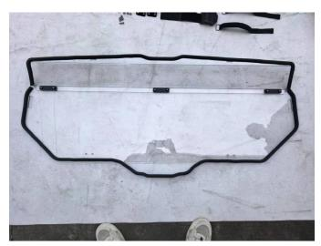
2. Put the rear windshield to the rear of the frame according to the position shown in the picture, and then fix the lower end of the rear windshield to the rear frame with four M6\*20 hex screws, four M6 lock nuts, and two brackets #5 and two brackets #6. As shown in picture:
