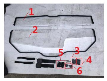
1. Assemble the PC board using six M6\*20 hex screws, three brackets #3, and three brackets #4. Install brackets #3 on the outside. As shown in picture:
