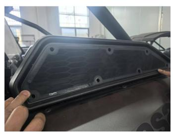
2. Install the air intake cover onto the filter screen using the removed plastic screws. As shown in picture:
