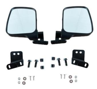
1. First, remove the 2 screws at the A-pillar of the original vehicle. Then, use the screws provided with the product to thread the bracket and lining tube onto the screws, and then re fix them back onto the A-pillar. Finally, use the matching screws and nuts to secure the reversing mirror to the bracket (the other side can be installed in the same way). As shown in picture:
