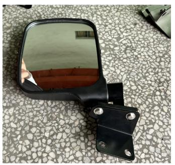
2. Unscrew the fixing screw at the A-pillar of the original vehicle, then use the screw that matches the side mirror, insert the aluminum lining tube, and install the side mirror bracket back onto the vehicle. Finally, use a nut to fix it (the other side can be installed in the same way). As shown in picture:
