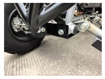
4. Fasten the center section of the skid plate with one M6x35 hex bolt, one M6 large flat washer (placed on top), one M6 small flat washer (placed below), and one M6 nut as shown in the diagram.
