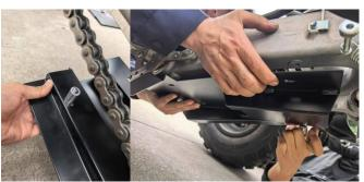
3. Secure the front end of the skid plate to the front frame using two M8x25 flange bolts with integrated washers as shown in the diagram.
