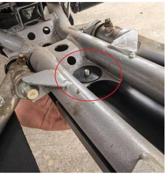
5. Fix the lower guard plate to the bottom of the frame with four M6x35 hex socket head screws and four M6 washers as shown in the diagram.
