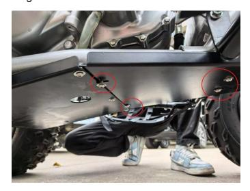
6. Fix both ends of the lower guard plate to the underframe of the vehicle using two mounting clamps and two M6x25 hex socket head screws. Finally, fully tighten all fasteners to complete the installation as shown in the diagram.
