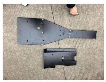
2. Mount component 4 to the rear chassis using four M6x40 hex socket head screws,
