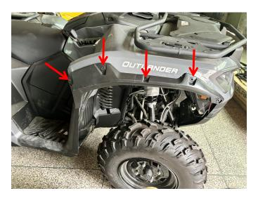
4. The rear fender flare can be installed following the same method as the front fender flare. First, position it in place on the vehicle. Then, using an M5 drill bit to drill holes in the vehicle body according to the screw holes on the fender flare. Finally, secure it with the
