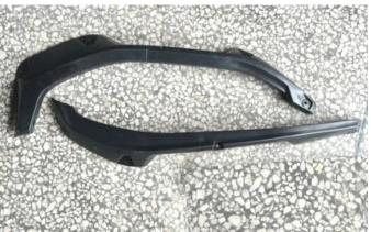
3. First, position the front fender flare in place on the vehicle. Then, using an M5 drill bit to drill holes in the vehicle body corresponding to the screw holes on the fender flare. Finally, secure it in place using the provided screws and nuts,
