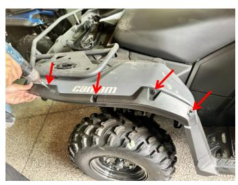
5. Finally, attach the rear mudguard by aligning it with the rear fender flare. First, secure it temporarily using the self-tapping screws. Then, using an M5 drill bit to drill holes in the vehicle body corresponding to the mounting holes on the mudguard. Complete the installation by fastening with screws and nuts for reinforcement. (The opposite side's front and rear fender flares can be installed following the same procedure.)
