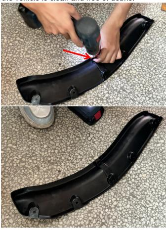
2. Place the assembled front fender flare in the corresponding position on the vehicle, then secure it using the included M6 self-tapping screws and flat washers. As shown in the figure:
