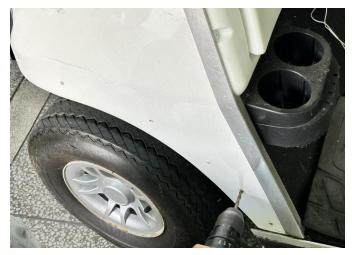
3. Place the fender flares back on the vehicle, and fix them in sequence with M6 screws and flat washer nuts. As shown in the figure:
