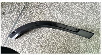
2. Install the assembled fender flare in place, then use an M6 drill bit to create holes in the vehicle body according to the mounting holes on the fender flare. As shown in the figure:
