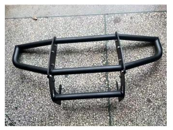
3. Install the two brackets (Part 5) onto the front bumper with six M6\*16 flange hexagon socket screws and M6 nuts.
