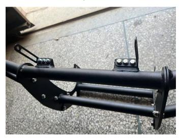
4. Use four M8\*20 flange hexagon socket screws and four M8 anti-loosening nuts to install the front bumper to both ends of the front frame, as shown in the figure. Tighten the screws and the installation is complete.
