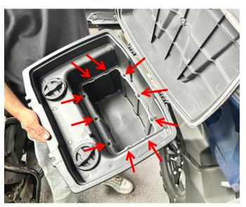
3. Insert the assembled storage box into the slots on the side rail of the rear cargo, then secure the storage box to the vehicle by twisting the two knobs inside the box. Finally, place the long storage compartment in the corresponding position of the storage box. As shown in the figure:
