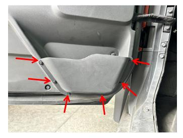
2. The rear door storage box is also installed and fixed in the same manner as above (the other side is installed in the same way).
